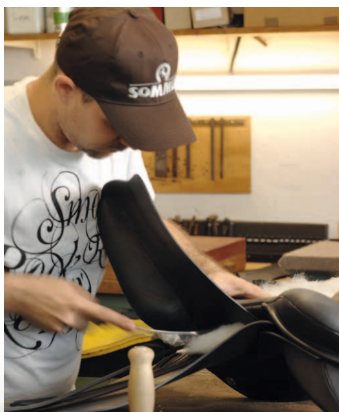
The saddle panels are filled with synthetic wool. Stuffing take place on the saddle itself.
