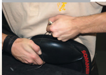
Hand-stitching the saddle panels
