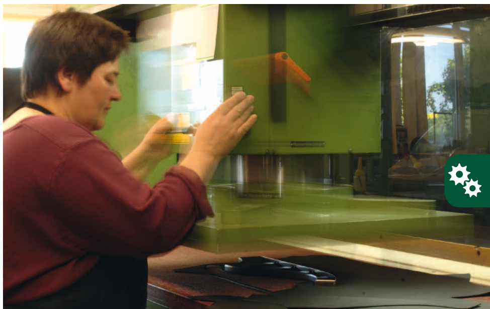
Stamping individual saddle parts, including quality control of the leather
